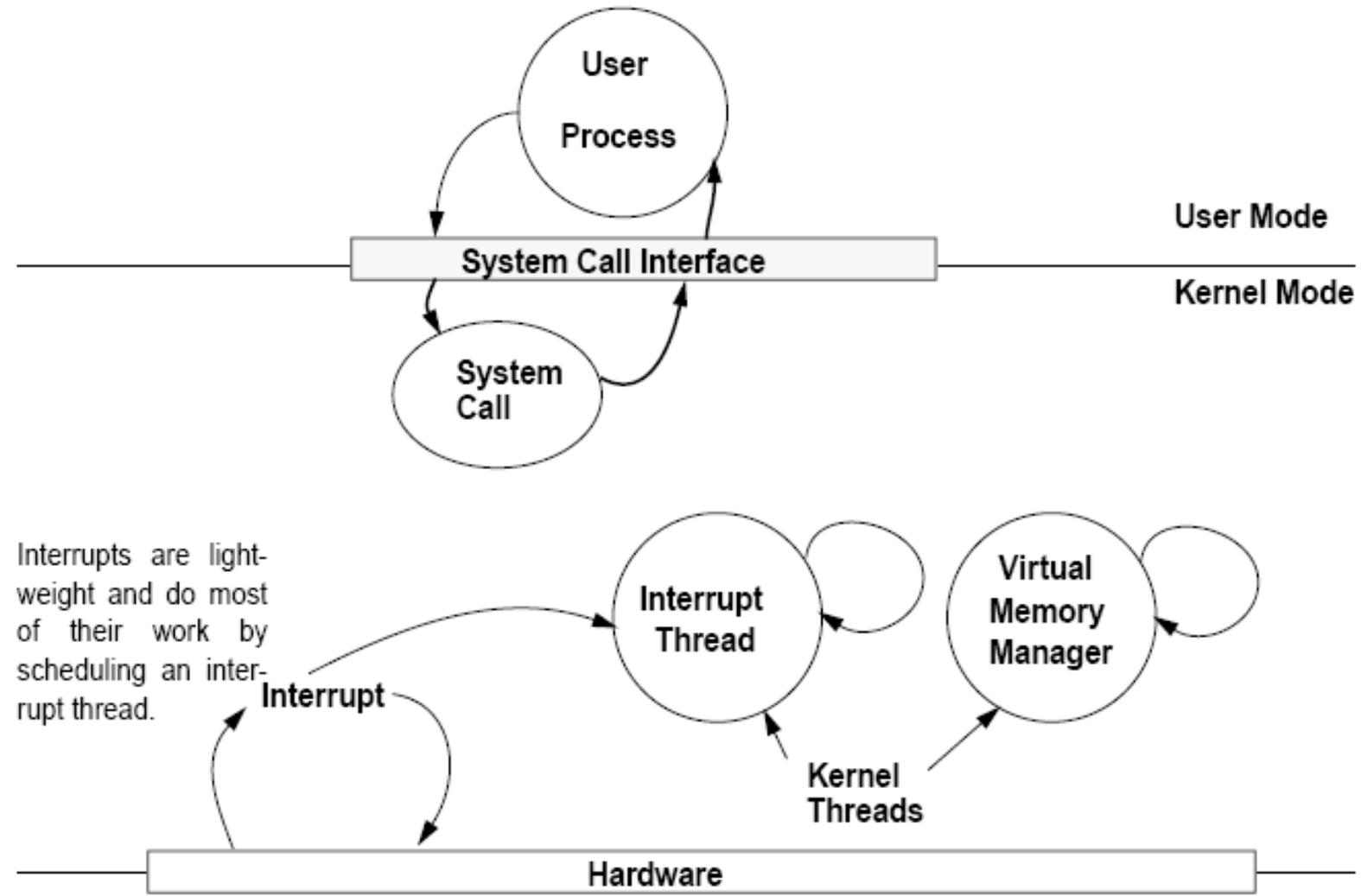
Interrupts are light-weight and do most of their work by scheduling an interrupt thread.
